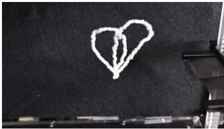
Figure 2: A levitating bead traced a heart-shaped-path along a user-defined hand gesture. The images of a video were added together to produce this LeviPainting.
